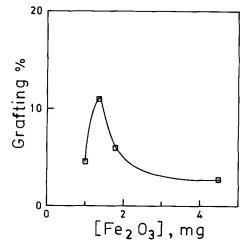
Figure 2 Variation of degree of grafting with concentration of colloidal  $Fe_2O_3$ . ([acrylamide] = 1 M)
