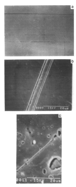
Figure 1 Scanning electron micrographs of ungrafted and grafted cellulose acetate films. (a) Ungrafted film; (b) acrylamide grafted film with simultaneous irradiation; (c) acrylamide grafted film with preirradiation process (magnification  $2000 \times$ )
